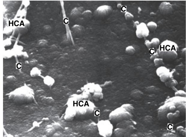
**Fig. 2.** Scanning electron micrograph of bioactive glass surface. Hydroxycarbonate apatite (HCA) mineral forming on the surface; collagen (C) fibres trapped into the HCA mineral, thus forming a biological bond.
