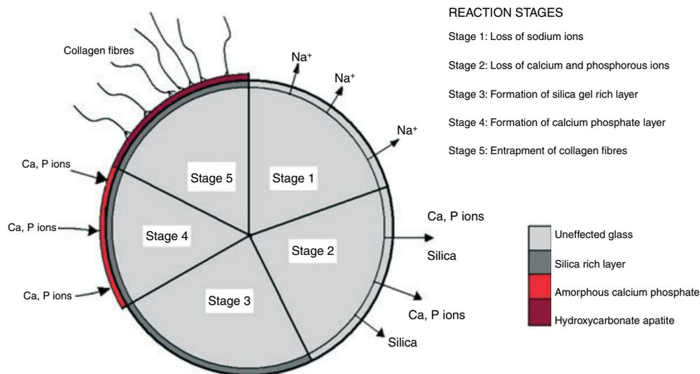
**Fig. 1.** Schematic diagram of bioactive glass reaction stages: (1) loss of sodium ions; (2) loss of calcium and phosphorus ions; (3) condensation to form silica gel rich layer; (4) amorphous calcium phosphate precipitates onto surface; (5) crystallization of amorphous calcium phosphate into hydroxycarbonate apatite, and thus entrapment of collagen fibres.
